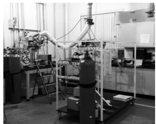
Water Gas Shift Skid
